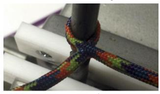
At this point I insert a <sup>1</sup>/<sub>4</sub>" drill bit into the loop just created to hold the loop size while I work.
